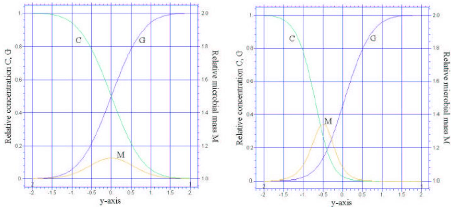
Figure 3. Electron acceptor C, contaminant G and microbial mass M distribution for  $Pe^T = 5$  and, left,  $M_C = 0$ ,  $M_G = 0$ ,  $L_\mu = 1$  and  $L_d = 1$ ; right,  $M_C = 0.5$ ,  $M_G = 5$ ,  $L_\mu = 5$  and  $L_d = 0.5$ .  $K_C$  and  $K_G$  equal unity in both cases.
