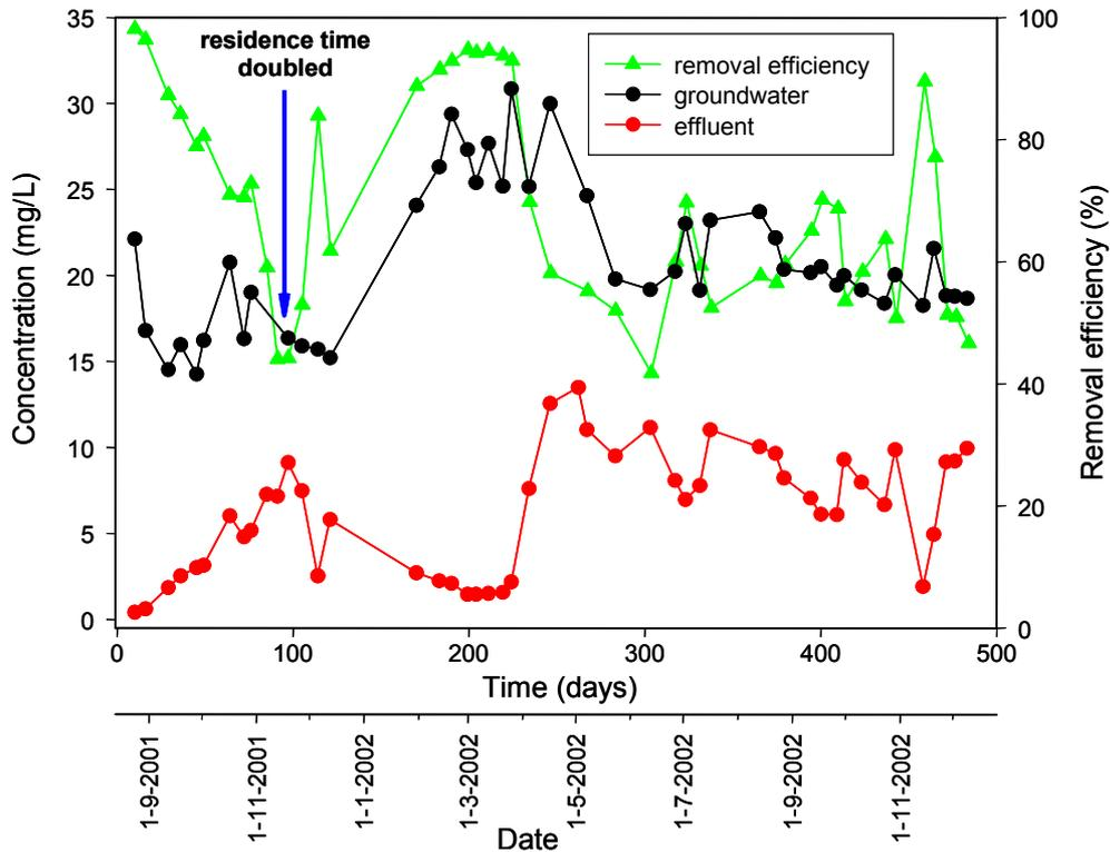
Fig. 37. Concentration of chlorobenzene and removal efficiency in microaerobic column 1 after its transfer to Bitterfeld. The residence time was doubled on day 99.
