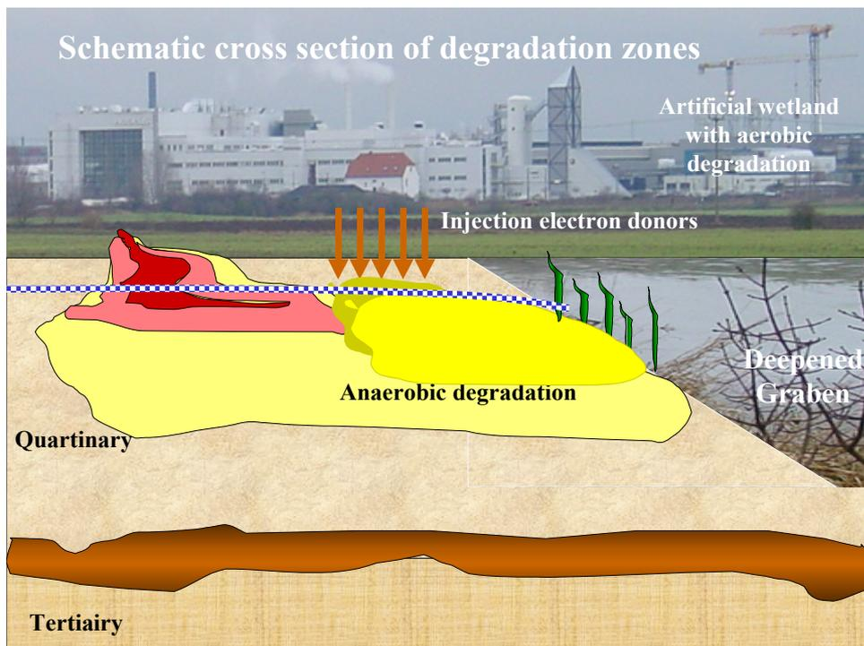
Fig. 52. Cross section of the anaerobic degradation zone with electron donor injection, and the artificial wetland in which aerobic degradation takes place (picture B. Satijn).
