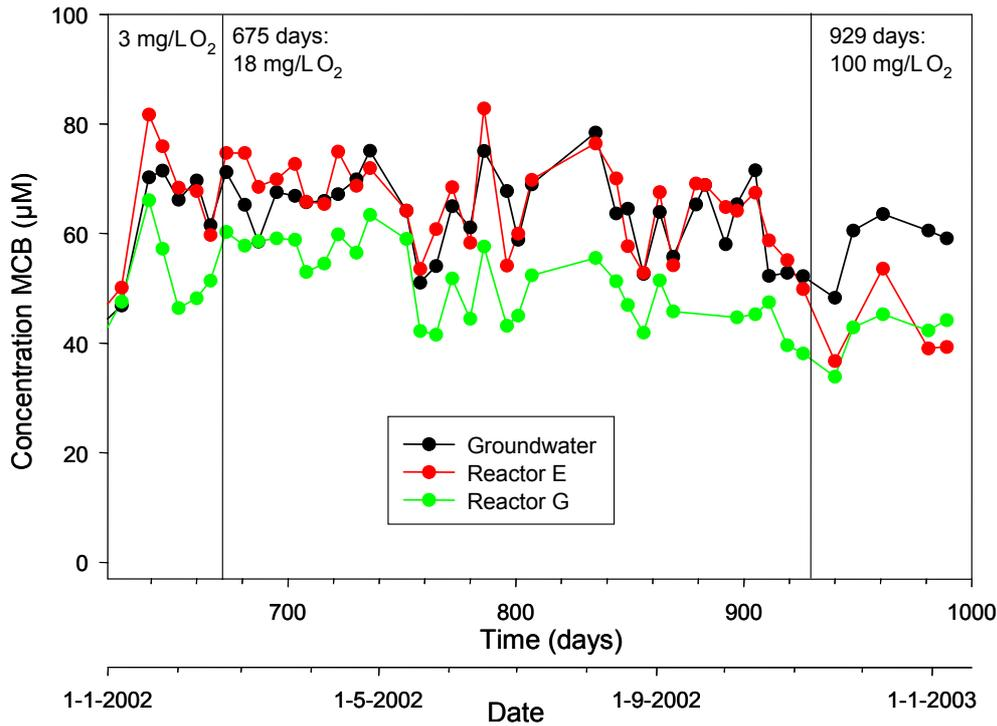
Fig. 46. Chlorobenzene concentrations in reactors e and g in 2002, after the hydrogen peroxide addition had been increased.
