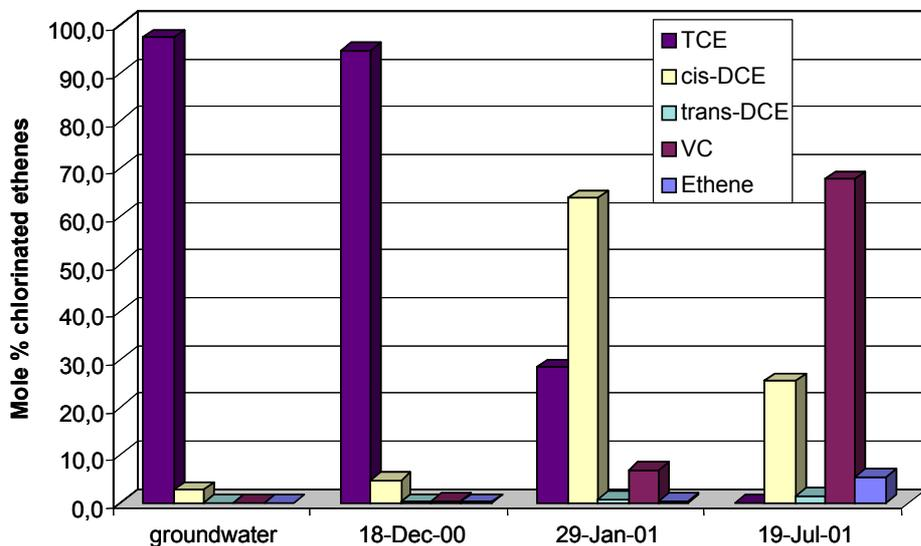
Fig. 30. Chlorinated ethenes contents of the influent (groundwater) and the effluent (on different dates) of the soil column with VFA/NH<sub>4</sub>Cl as e-donor/nutrient.
