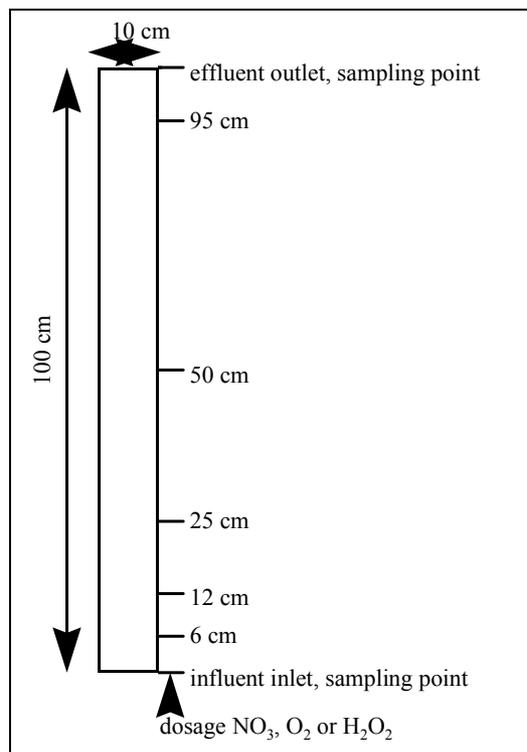
Fig. 16 Set-up of micro-aerobic column.
