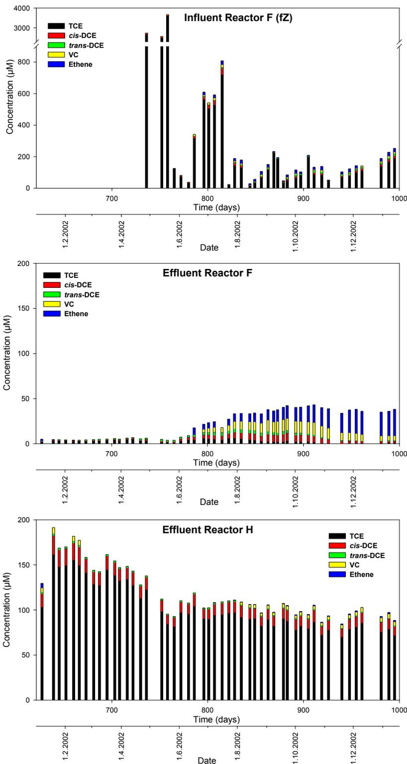
Fig. 43. Anaerobic transformation of chlorinated ethenes in reactor system II (reactors f and h) after the change of the electron donor addition in February 2002.
