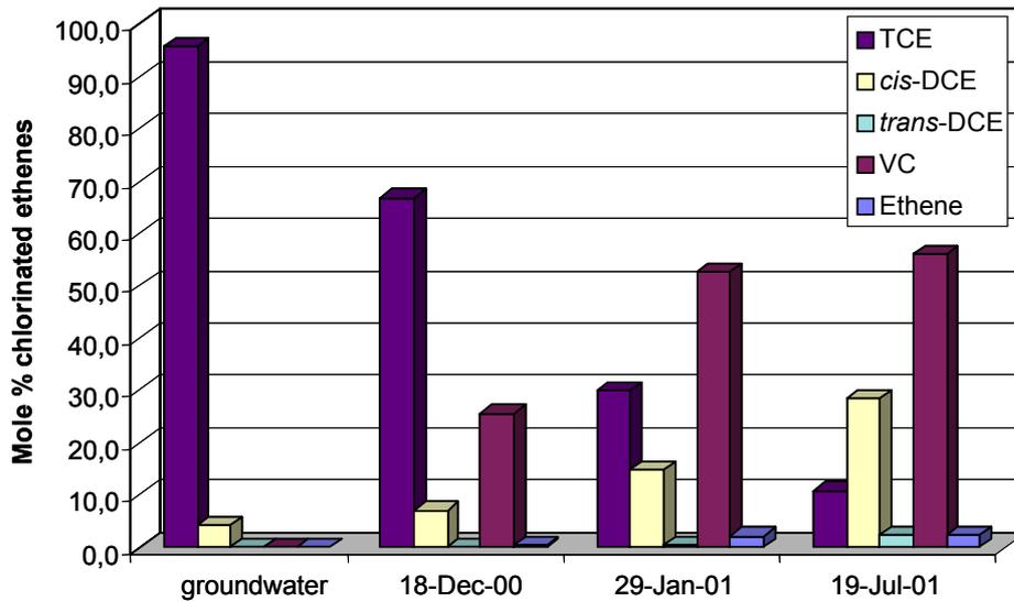
Fig. 29. Chlorinated ethenes contents of the influent (groundwater) and the effluent (on different dates) of the soil column with methanol/G31 as e-donor.
