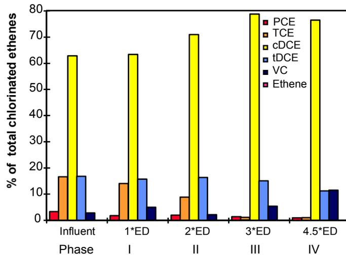
Fig. 27. The effect of increased electron donor concentration on the transformation of TCE in the Bitterfeld groundwater.
