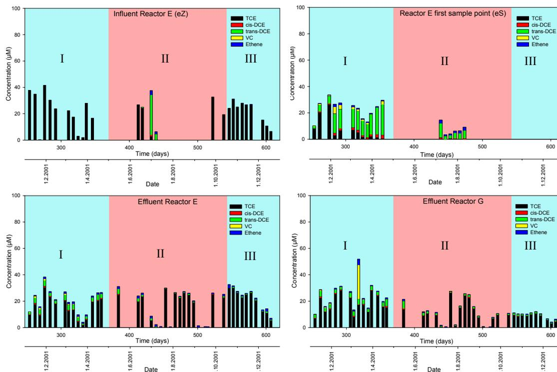
Fig. 41. Transformation of chlorinated ethenes in reactor system I: reactors e (anaerobic) and g (microaerobic). The colored time periods mark the normal operation of the reactors (I), operational problems (clogging, excessive gas production)(II), and the discontinuation of the electron donor supply (III).
