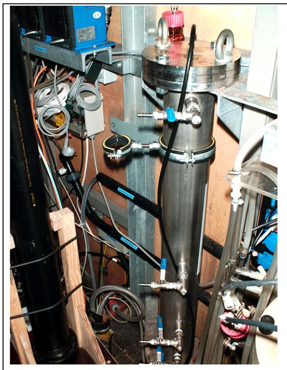
Fig. 17 The micro-aerobic column in the mobile on-site test unit.
