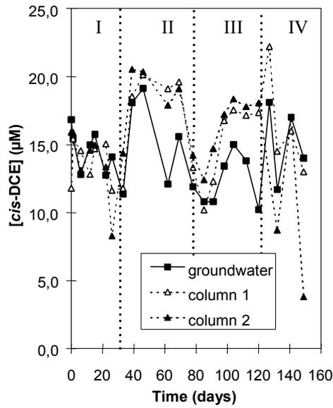
Fig.24 Transformation of cis-DCE in the anaerobic columns treating the groundwater from Bitterfeld.
