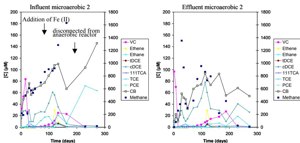
Fig. 35. Concentration of chlorobenzene and lower chlorinated ethenes in micro-aerobic column 2 (30-98 R).
