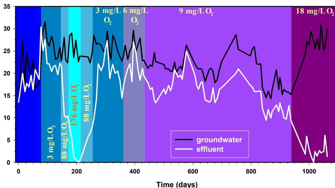
Fig. 36. Influent (groundwater) and effluent concentrations of the on-site micro-aerobic column. The column was operated with 2.4 mM NO<sub>3</sub> in the influent and oxygen concentrations as indicated in the graph.
