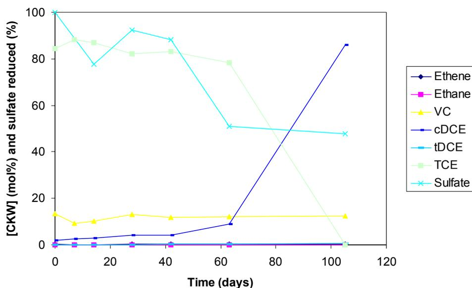
Fig. 19. Reduction of sulphate and TCE at low electron donor (0.1 ED as acetate) concentration.
