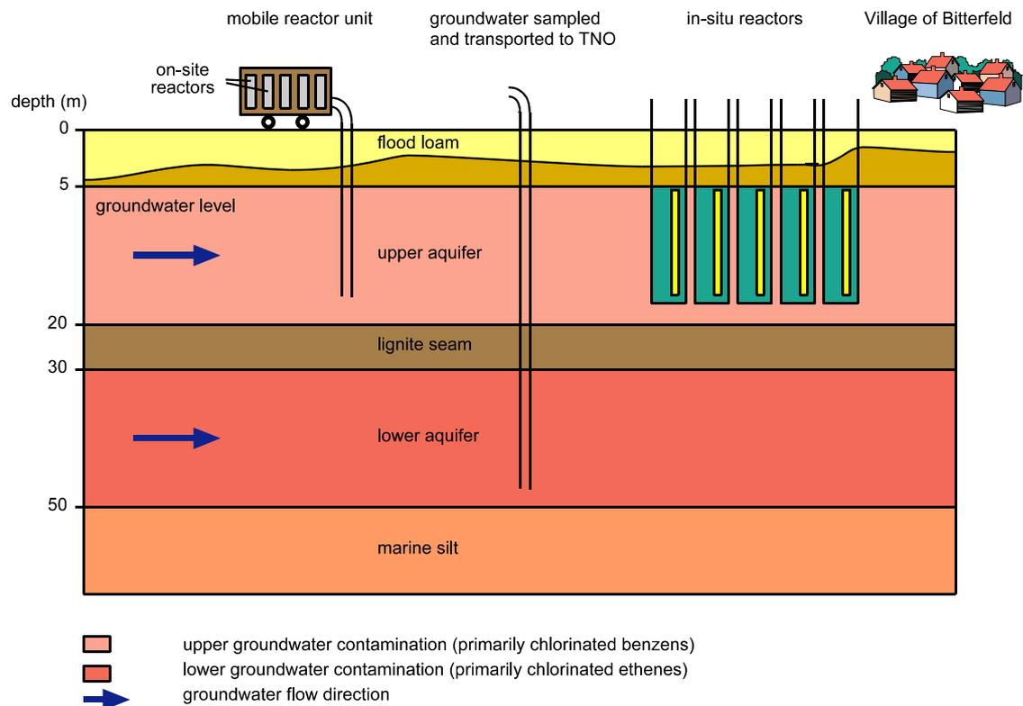
Fig. 4. General set-up of the on-site mobile test unit.
