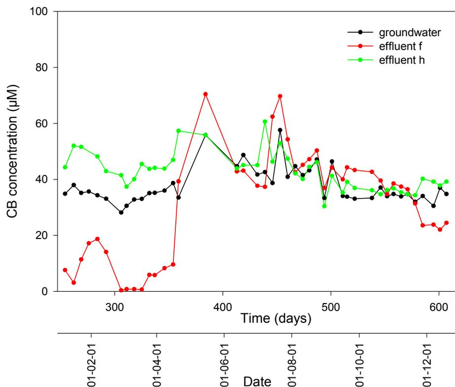
Fig. 45. Concentration of chlorobenzene in groundwater and anaerobic and microaerobic effluent (reactor system f-h).
