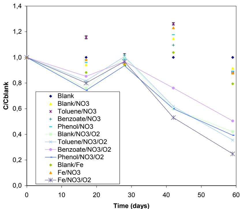
Fig. 20. Chlorobenzene concentration relative to the concentration in blanks without any addition (Cblank) given in time.
