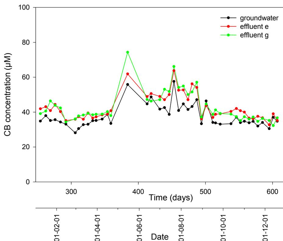
Fig. 44. Concentration of chlorobenzene in groundwater and anaerobic and micro-aerobic effluent (reactor system e-g).
