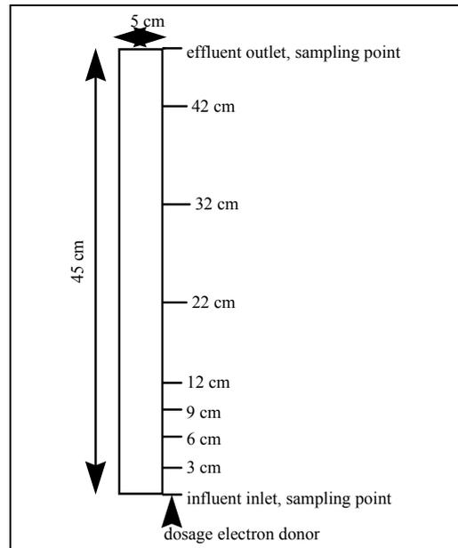
Fig. 14. Set-up of anaerobic column.
