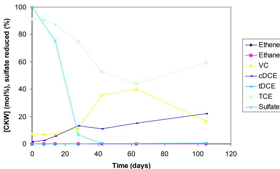
Fig. 18 Reduction of sulphate and TCE in high electron donor (10\*ED, MeOH/G31) concentration batches.
