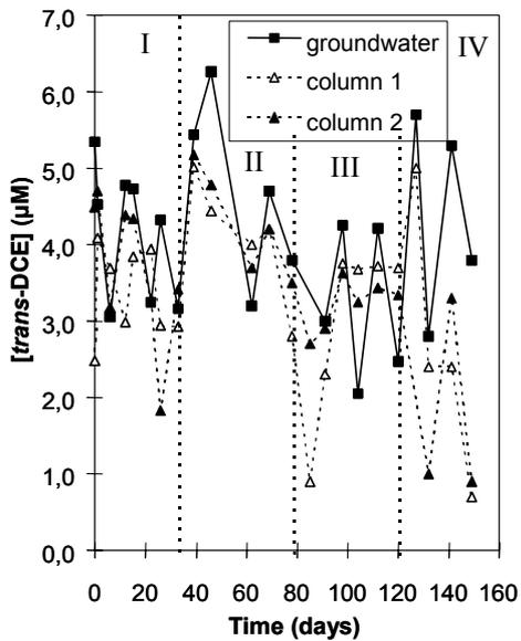
Fig. 25 Transformation of trans-DCE in the anaerobic columns treating the groundwater from Bitterfeld.
