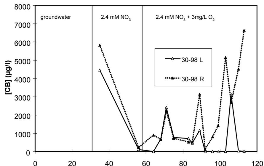
Fig. 31. Chlorobenzene removal in two micro-aerobic laboratory column systems.
