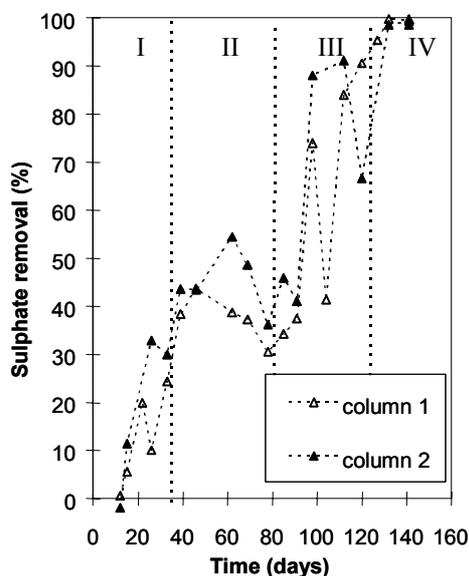
Fig. 21 Sulphate reduction in the anaerobic column treating the TCE containing groundwater.
