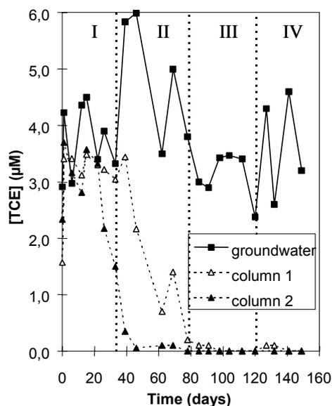
Fig. 22 Transformation of TCE in the anaerobic columns treating the groundwater from Bitterfeld.
