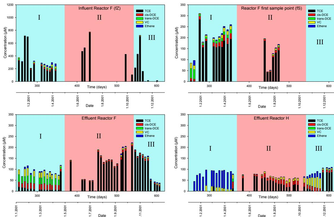
Fig. 42. Transformation of chlorinated ethenes in reactor system II: reactors f (anaerobic) and h (microaerobic). The colored time periods mark the normal operation of the reactors (I), operational problems (clogging, excessive gas production)(II), and the discontinuation of the electron donor supply (III). N.B. Please note the difference in concentration scale between the upper left graph and the other graphs.
