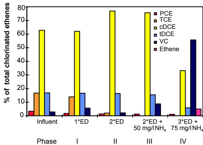
Fig. 28. The effect of increased electron donor concentration and the addition of nitrogen on the transformation of TCE in the Bitterfeld groundwater.
