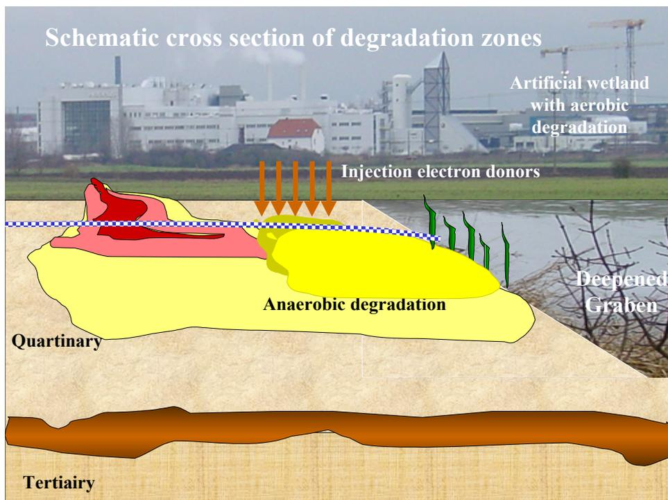
Fig. 47. Cross section of the anaerobic degradation zone with electron donor injection, and the artificial wetland in which aerobic degradation takes place.
