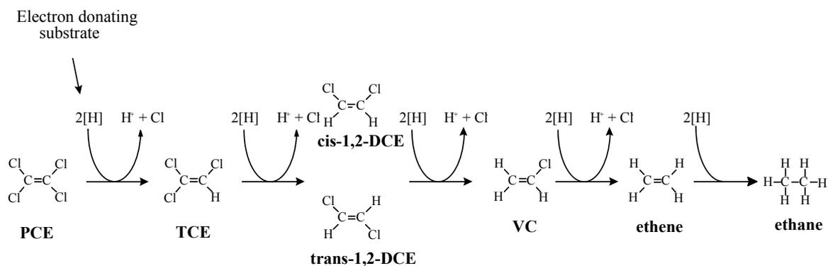
Fig. 8. Complete reductive dechlorination of PCE and TCE under anaerobic conditions.
