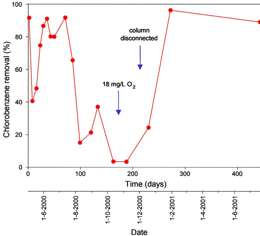
Fig. 33. Chlorobenzene removal in microaerobic column 30-98 L. The influent concentration fluctuated between 7-11 mg l<sup>-1</sup>. On day zero, this column received 0.24 mg l<sup>-1</sup> potassium nitrate and 3 mg l<sup>-1</sup> oxygen in the influent. On day 169, the oxygen concentration was increased to 18 mg l<sup>-1</sup>. On day 219, the column was disconnected from the anaerobic column.
