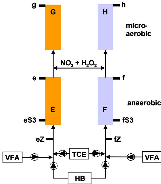
Fig. 38. Schematic set-up with additions and sample ports of the *in situ* reactor systems.
