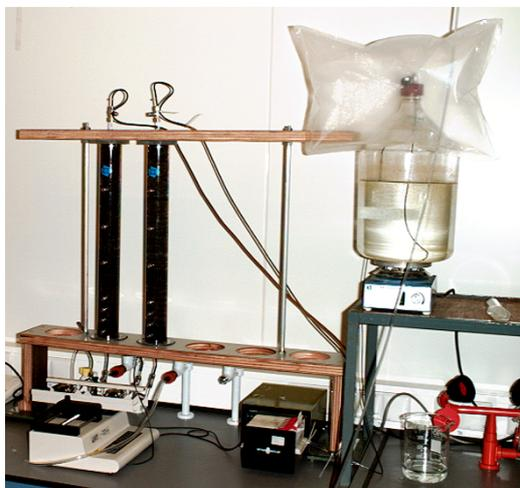
Fig. 15. Set-up of the anaerobic columns.
