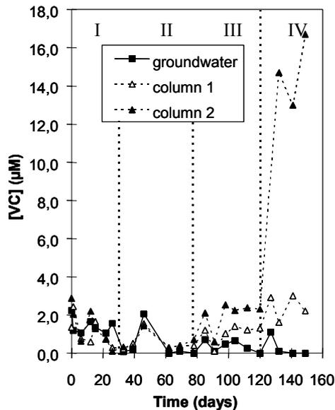
Fig. 26 Transformation of VC in the anaerobic columns treating the groundwater from Bitterfeld.
