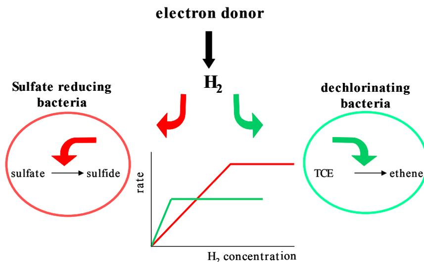
Fig. 12. Flow of electrons to sulphate reduction and dechlorination and the effect of hydrogen concentration on the reduction rate of sulphate and TCE.
