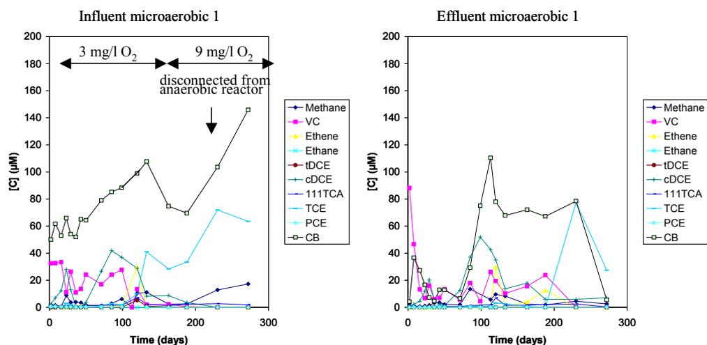
Fig. 34. Concentration of chlorobenzene and lower chlorinated ethenes in micro-aerobic column 1 (30-98 L).
