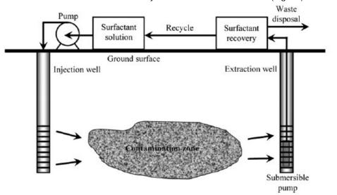
Fig. 18: General scheme of the pump and treat method for remediation of a contaminated site (Paria, 2008).
