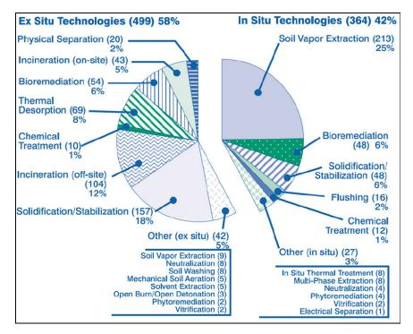
Fig. 17: Technologies selected for source control at superfund remedial action sites from 1982–2002 (Paria, 2008).
