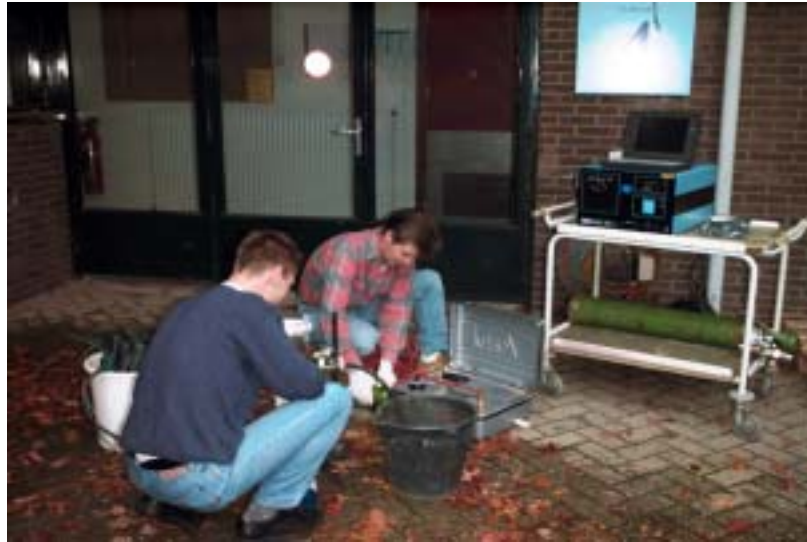
Fig. 12. Measuring hydrogen in the field, with the GC-RGD on a trolley.
