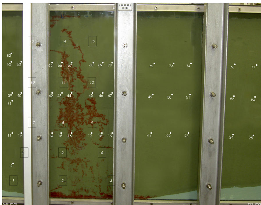
Figure 6.7: Picture on day 0, PCE formed in an irregular residual zone with a pool at the bottom.
