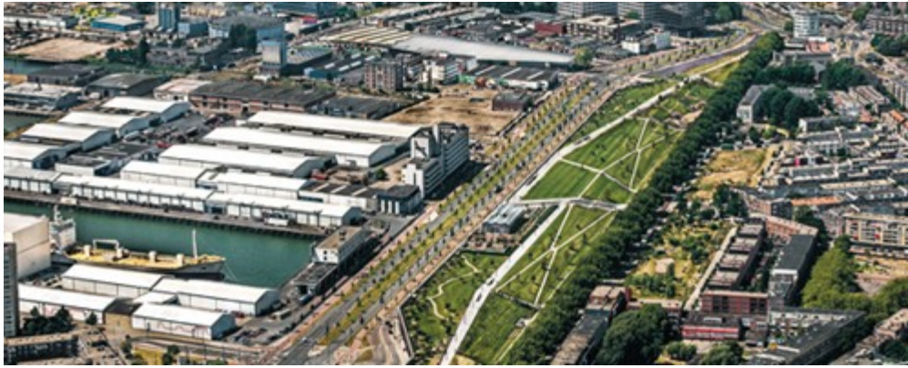
Figure 6.6. On a former shunting-yard has in 2013 the Roof park Rotterdam opened, the larger roof park of Europe. By applying green area on the rooftop of shopping malls, 80.000 m 2 of park is added to the city (Schaeken et al, 2014).
