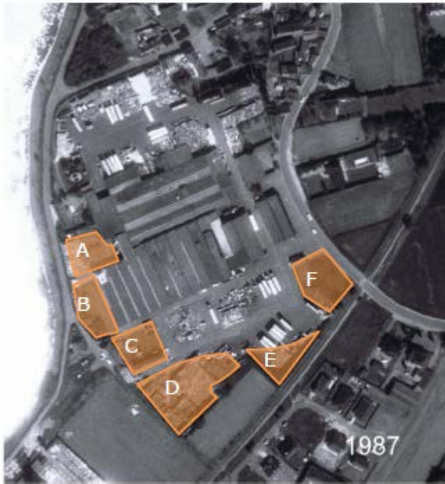
Figure 6.14. Aerial view of 1987 indicating potentially suspicious zones (A: processing liquid waste; B: processing (liquid) waste and burn-out of containers, C: processing liquid waste (above-ground and underground tanks), D: processing empty containers and burn-out of containers and E: Landfill.
