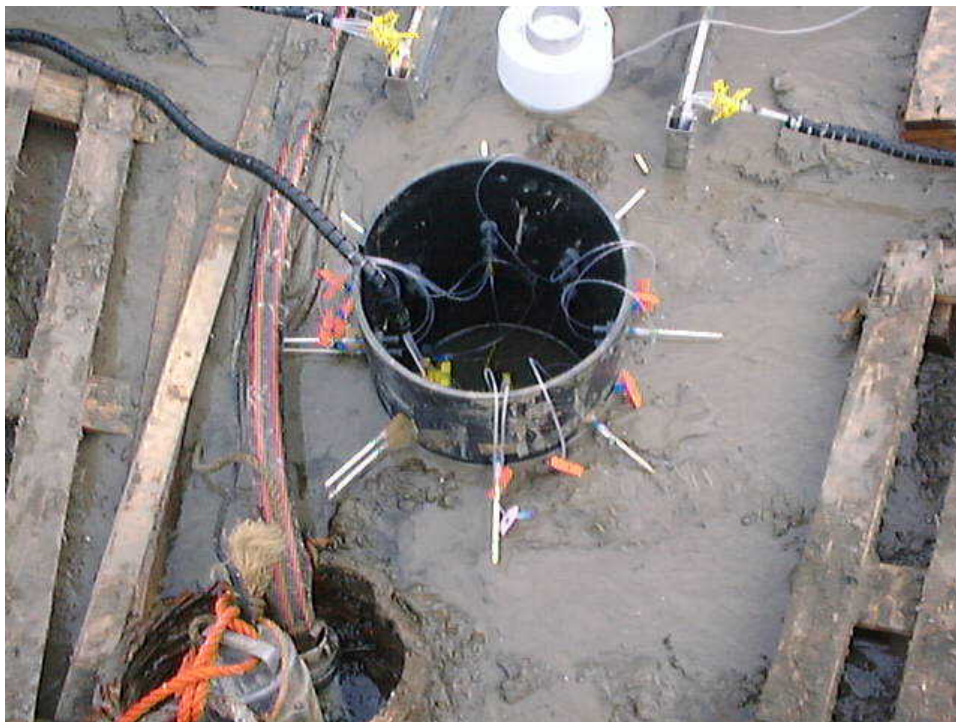
Fig. 10. Top view of the main tube, inserted into the sediment. The small filter tubes are pushed from inside into the sediment.
