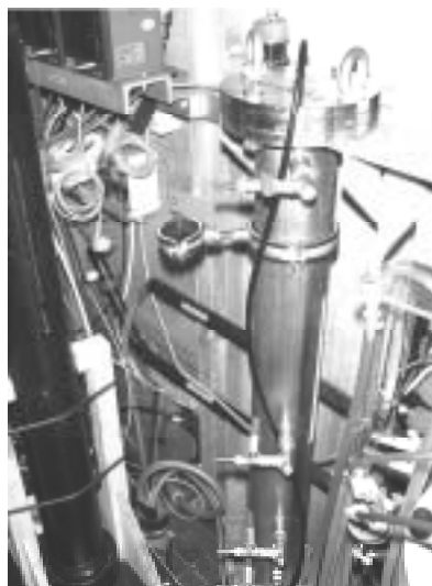
Fig. 13. The microaerobic column in the mobile on-site test unit.
